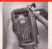
3. Break the film seal and pull the end of the paper (colored side up—black side facing the lens) to the take-up spool. Thread the paper as far as it will go into the longer slot of the take-up spool, pull out the winding knob as far as it will go, and turn it twice to bind the paper on the spool.
