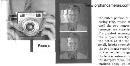
LOOK through the eyepiece of the combination viewfinder and rangefinder with the camera pressed firmly against the face. Select any vertical line in your subject as seen in the bright rectangle in the finder, and with your finger on
