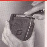
1. Press the latch down firmly with the ball of the index finger; then move the back lock down toward the bottom of the camera by pressing with the thumb against the end of the slide. Swing the back out to about a 90° angle with the camera and lift it off.
