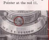
C-Set the Focus\* Set the Focusing Ring so the red 10 is at the black index mark. With Kodachrome Film Daylight Type, the shutter speed at 50, and lens opening at the red dot, your subject must be between 71/2 and 16 feet from the camera: with Kodak Plus-X Film (lens opening at 11), your subject must be between 6½ and 30 feet from the camera to be in focus. \*The rangefinder method of focus is described on page 11.
