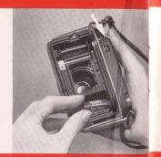
2. If the empty take-up spool is not in the winding knob (arrow) end of the camera, place one end of the empty spool on the winding key center and drop the other end into its recess. Place the film in the end opposite the winding knob so that the paper will draw off the top of the roll.
